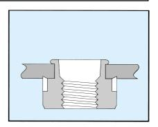
Support bush from base and drive punch into counterbore riviting the spigot over onto the parent material until almost flush
