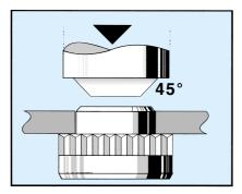
Locate knurled spigot in hole so that shoulder resting on surface of parent material and knurl protudes through to the other side
